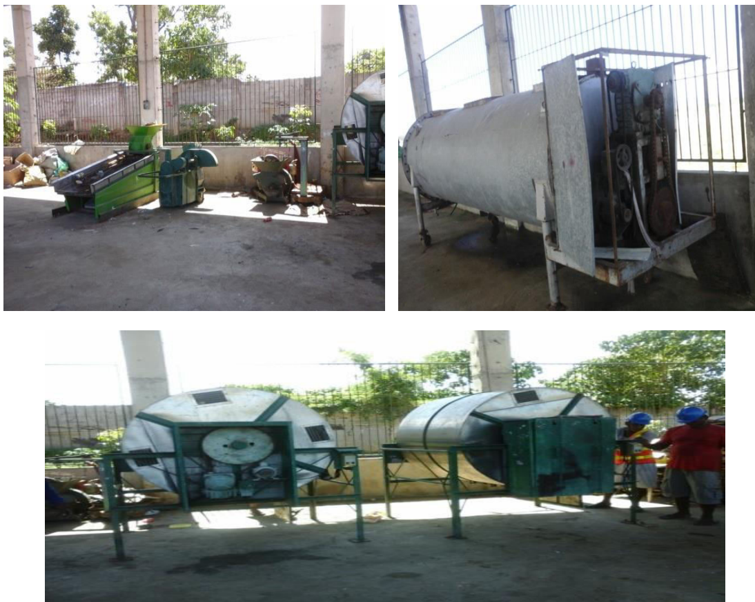
Rotating drums and bioreactor for City MRF
